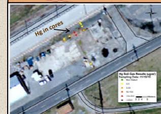
Hg retort building 81-10 – Known Hg spills and Hg beads observed in cores. Soil vapor data suggests the extent of elemental Hg spill has not been defined to the north.
