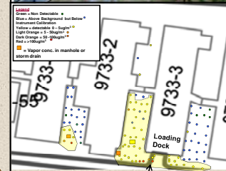
9733 Engineering building – Hg beads observed during excavation activities in an area used as a loading dock for Hg.
