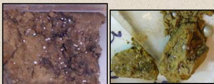
Hg beads in soil cores collected from the Building 81-10 former Hg retort facility
